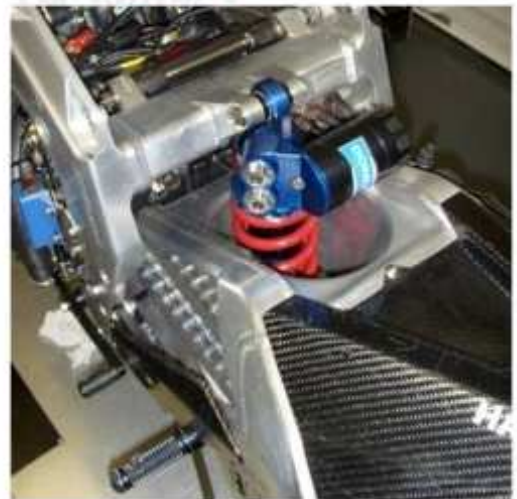
The Zenium damper mounted on the Suter bike - 16/12/2010
