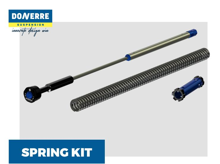
Spring kit for full-size KTM SX & SX-F models and Husqvarna TC & FC models replacing the original WP AER cartridge. Spring preload is adjustable from the outside with indexing. Our Spring Kit is fitted with a thrust needle roller bearing to reduce spring friction for better handling.
